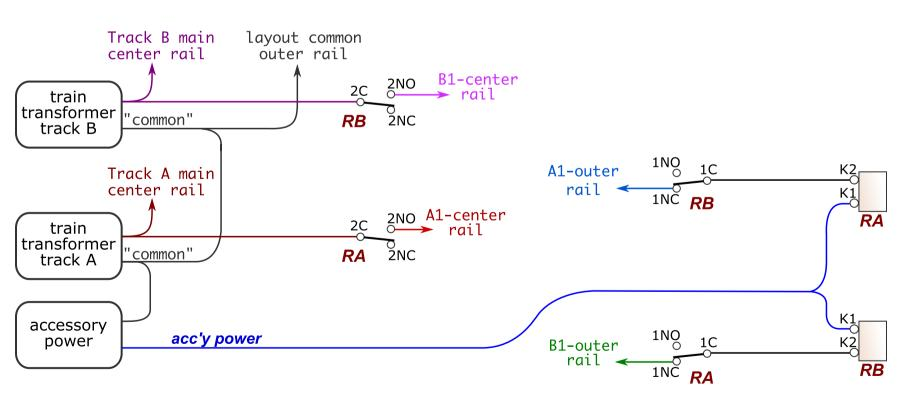
'RA' and 'RB' are two double-pole (DPDT) relays, such as Azatrax MRAPR-12v.
