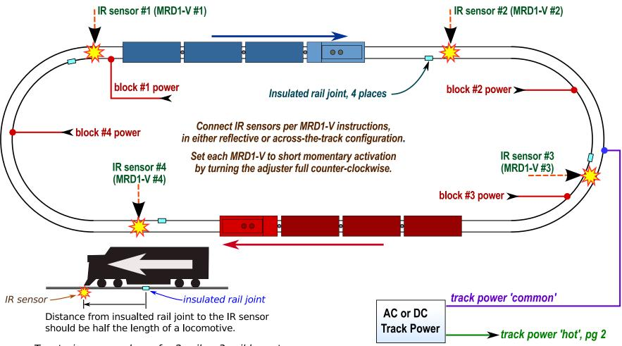
Two trains on one loop, for 2-rail or 3-rail layouts. Note: For 3-rail track, the insulated rail joints and the block power connections are on the center rail. Track power 'common' connects to the outside rail.
