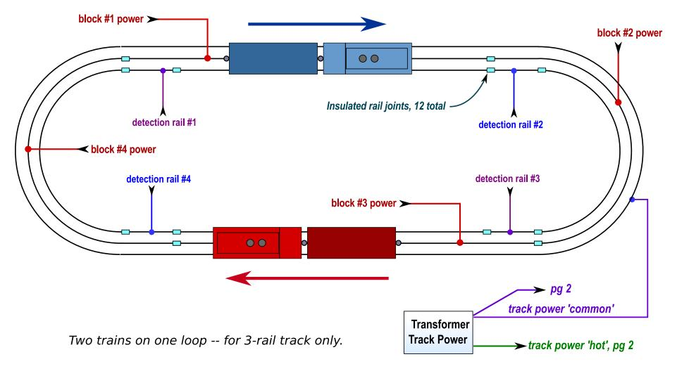
As a train enters a block, it trips a relay that turns off power to the block that is behind the locomotive. It also trips another relay that turns power back on to the second block behind the locomotive.
