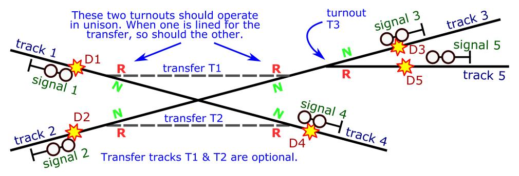
Azatrax TS5-Xing. An Azatrax MRD1-NV is needed for detector D5. Turnout T3 is always on track3. Turnout T4 is always on track 4. Use one, not both. Note the placement difference of T3 vs. T4, relative to the transfer track turnout.
