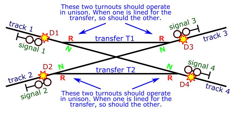
Transfer T1 always connects with track 1 and track 3. Transfer T2 always connects with track 2 and track 4.
