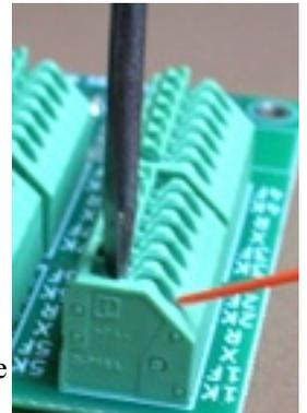
**Connect sensor set 1:** Connect the red wire from the IR LED to terminal 1K. Connect the blue wire from the IR receiver to terminal 1F. How you connect the white and yellow wires to the D6X will determine whether Detector 1 will operate in 'Across the Track' or 'Reflective' mode. See the diagrams below.
