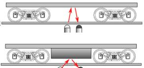
Angling the IR LED and receiver toward each other is best for N and HO scale where the trains are close to the rail head, and in places where an object above the track might otherwise cause false detections. Angle the
