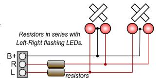
LED signals must have resistors wired in series to limit the LED current. A resistor may be wired in series with the L and R signal wires (two resistors total). Or one resistor may be wired in series with the 'base' ('common') signal wire.
