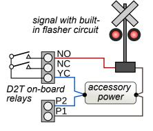
The contact of the 'normally closed' relay is connected to terminals 'YC' and 'NC.' This relay is 'on' when the signals are off. Terminal 'YC' is common to both relays.
