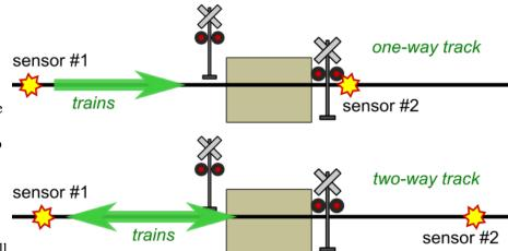
turn off. If the end of a short train clears the first sensor before the front of the train reaches the second sensor, the signals will stay on for 12 seconds to give the train time to reach the second sensor.
