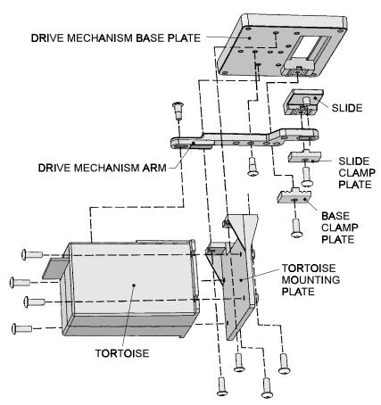
Check to make certain that there are no obstructions on the underside of the layout. There must be at least 1/4" clearance between the center of the hole you just drilled and the nearest obstruction. You will also need adequate clearance below the underside of the layout to drill pilot holes and drive the screws through the Actuator Mounting Plate up into the underside of the layout.
