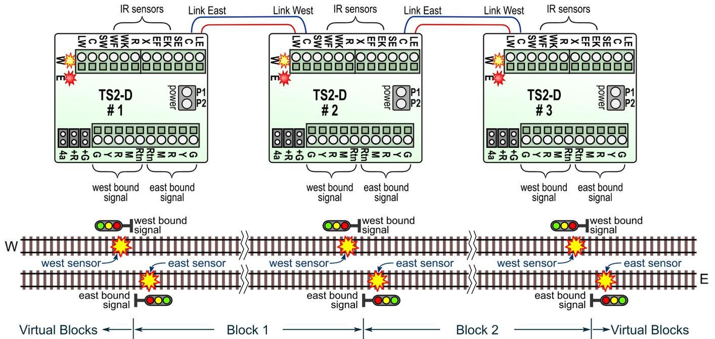
**The TS2-D may be linked to other TS2-D circuits** to the east and/or west. The TS2-D circuits tell each other when they sense a train entering or leaving the block between them. When a train enters a block, the block is 'occupied' until a train exits the block. The block is then considered to be 'clear.'
