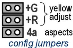
Two configuration jumpers (small rectangular connector blocks, or 'shunts') are supplied with the TS2-D. Three pairs of pins can accept these jumpers. To enable a configuration feature, place a jumper across both of the pins. To disable a feature, remove the jumper or park it on one pin.
