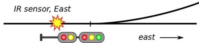
**For example** – a turnout is to the east of a dual head signal. The 2-light lower signal head indicates the position of the turnout points.
