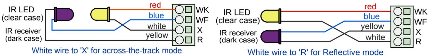
Additional wire may be spliced to the sensor leads if needed. Use similar twisted pair wire for total length up to 26 ft (8m).
