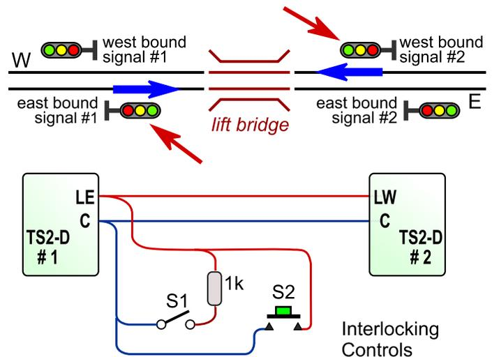
**To manually clear an 'occupied' block,** momentarily connect the 'Link' terminal (LE for the east side, or LW for the west side) directly to the 'C' terminal. This may need to be done after a train leaves the block through a turnout onto a siding or branch line, or if it is removed from the track by hand. In this diagram, briefly pressing S2 will clear the block between TS2-D #1 and TS2-D #2.
