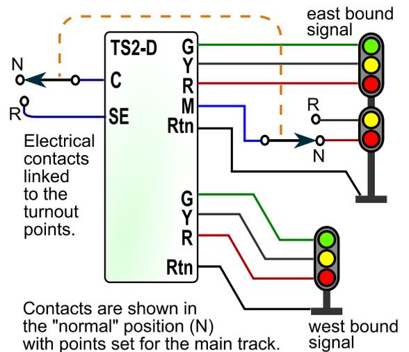
The two sets of electrical contacts are linked to the switch machine. These can be internal contacts such as are built in to Tortoise® and Cobalt® switch machines, or they can be contacts of a latching relay that operates in parallel with the switch machine.
