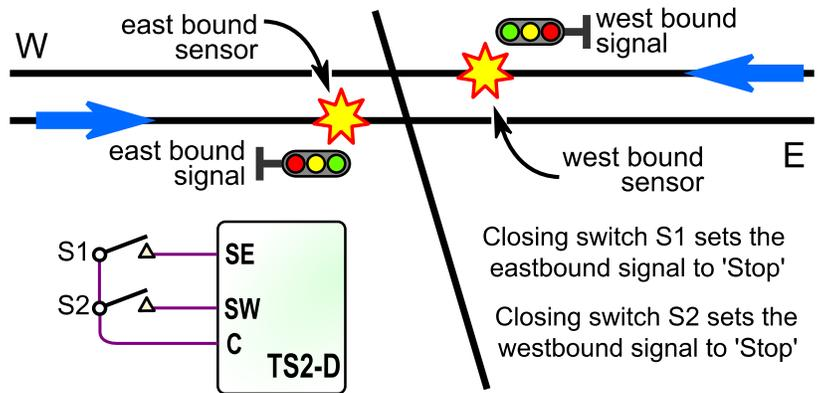
**To force either signal to a 'stop' condition,** rather than for an entire block as shown above:
