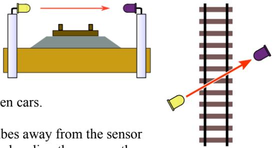
**Tip #2** - If mounting the sensors vertically as shown here, slide the plastic tubes away from the sensor then carefully bend the leads to a right angle. The leads are somewhat brittle, bending them more than two or three times may cause a break.
