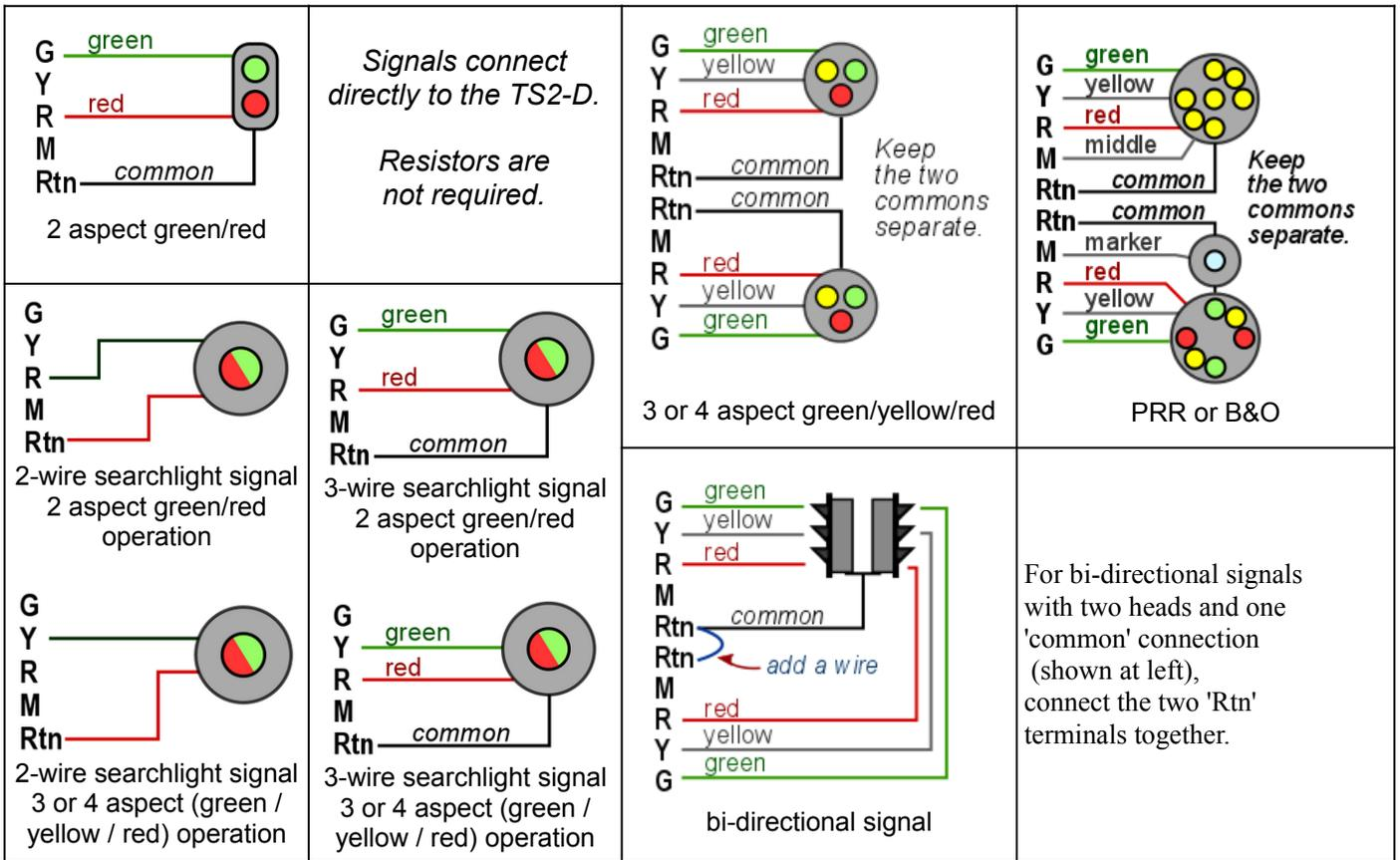
Note that **resistors are not required** because resistors are built in to the TS2-D circuit board. If signals are pre-assembled with resistors, first try the signals with their resistors. If the signal lights are too dim, remove the resistors.
