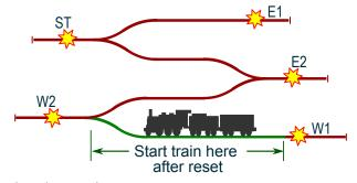
If it does not move at all, change the direction switch on the power pack and try again. If the train moves in the wrong direction, swap the track power wires at terminals main N and main S.
