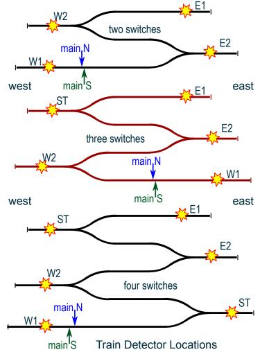
**ST** detectors cannot be used at the top or bottom terminal tracks (E1 or W1).
