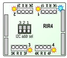
Pins used: A4 & A5 for I2C communication, +5v and ground. All other pins are pass-through only.
