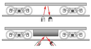
For N and HO scale and where the object to be sensed is close to the IR LED and receiver, mount the IR LED and its receiver so they are both pointing at the same spot on the object. Angle the IR LED and photo
