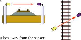
**Tip #1** - If mounting the sensors vertically as shown here, slide the plastic tubes away from the sensor then carefully bend the leads to a right angle. The leads are somewhat brittle, bending them more than two or three times may cause a break.
