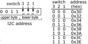
**Read registers:** To learn what is happening within the RIR4, the master reads data from the RIR4 read registers. The master first sends the RIR4's I2C device address onto the I2C bus. This gets the attention of the RIR4.
