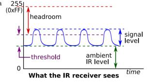
**Detector sensitivity:** The detector circuit is looking for variations in the received IR light that match the pulses transmitted by the IR LED. The received pulses ride on top of the ambient IR level. When the
