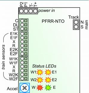
The PFRR controller has connections for up to two train sensors. They are numbered W1, W2, E1 and E2. **The operating mode of the PFRR is determined by the combination of sensors that are connected.** So be careful to connect your sensors to the correct terminals on the PFRR controller. The wrong combination will result in unexpected operation.
