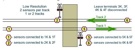
right to left, encountering sensor 5 first. If trains travel in both directions on track 1, place the two sensors equal distances from the crossing. Sensors 2 and 6 on track 2 operate in the same way as the sensors on track 1.
