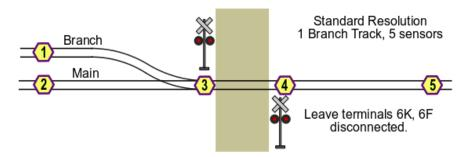
Single Track Crossing, One Turnout - This operates in 'standard resolution' mode because four sensors are used for each possible path that a train can take through the crossing.
