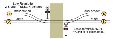
**Two Turnouts** - This operates in **'low resolution'** mode because two sensors are used for each possible path that a train can take through the crossing.
