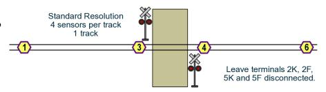
the train clears both sensor 3 and sensor 4 the signal will turn off. Similar operation occurs when a train travels right to left.
