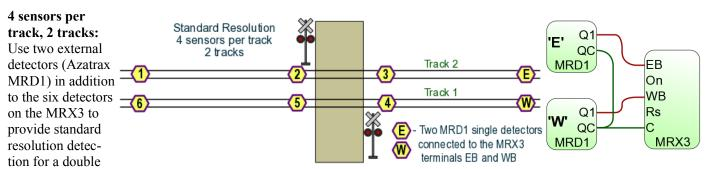
track crossing. Install the two single detectors according to their instructions, and connect them to MRX3 terminals 'EB' and 'WB' as shown. Each track is independently monitored in the same fashion described above for '4 sensors single track.'
