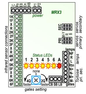
show the status of the detectors -- 'on' if the circuit is detecting an object, 'off' if no object is detected. External train detectors, such as current sensing block detectors may also be used with the MRX3. See page 6. Signals can have left/right flashing lamps and/or non-flashing lamps. Operating crossing gates are supported in either 2quadrant or 4-quadrant configuration (see pg. 5). The MRX3 also has connections for triggering an external sound module or other accessories (see pg. 6).
