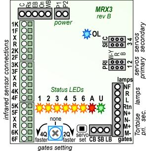
turn the adjuster back gradually. The yellow LEDs will successively indicate lower gate speeds. Slowest gate speed is 1. In 4-quadrant operation, gates connected to the 'primary' connections will close before the 'secondary' gates close. When the crossing clears, the secondary gates open before the primary gates open.
