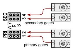
Only change connections to the MRX3 while power is off. Servo connectors can be tight. Always support the circuit board with your fingers when removing a servo cable.
