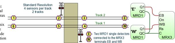
double track crossing. Install the two single detectors according to their instructions, and connect them to MRX3 terminals 'EB' and 'WB' as shown. Each track is independently monitored in the same fashion described above for '4 sensors single track.'
