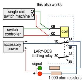
1,000 ohm resistor for LED signals
