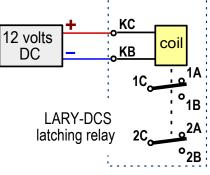
When the +/- polarity is reversed at KC and KB, the contacts will switch. Terminal 1C will
