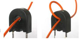
Connect each sense coil to the DBD2 module with twisted pair wire, such as from telephone or "Cat 5" ethernet cable. Keep the twisted pair away from track power wires to avoid inducing a false signal in the sense wires. If the twisted pair wires are kept away from track power and other digital signal sources, the sense coils can be placed as far as 12 ft (4 m) from the DBD2 module.
