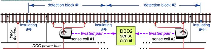
Each of the two detection blocks must have one rail electrically isolated from the rest of the layout. Cut an insulating gap in the rail or use plastic rail joiners at each boundary of the detection block.
