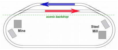
with identical empty cars. The loaded train travels from its hidden siding, around the producer site (coal mine) to the consumer site (steel mill) and then into the hidden area and its siding. The loaded train stops, then a few seconds later the empty train travels in the opposite direction from its siding, around the consumer site to the producer site, then behind the backdrop to its siding. After another pause the cycle repeats.
