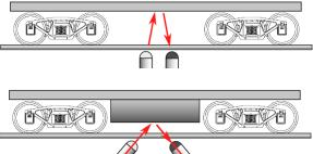
Angling the IR LED and receiver toward each other is best for N and HO scales where the trains are close to the rail head, and in places where an object above the track might otherwise cause false detections. Angle the
