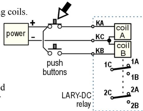
The contacts remain latched in this position after power is removed from the coil.
