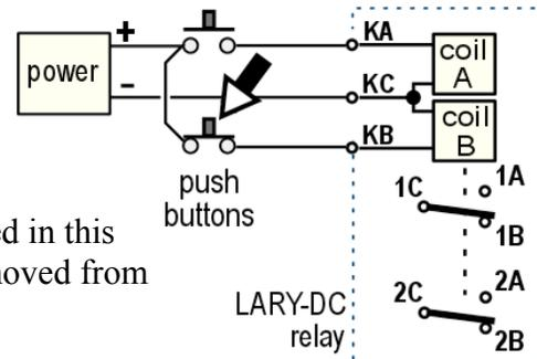
The contacts remain latched in this position after power is removed from the coil.
