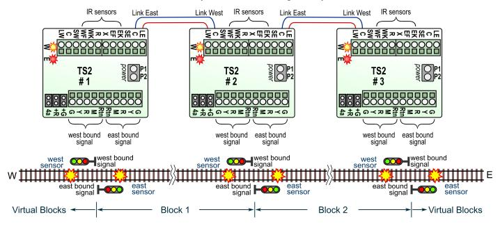
The TS2 may be linked to other TS2 circuits to the east and west. The TS2 circuits tell each other when they sense a train entering or leaving the block between them. When a train enters a block, the block is 'occupied' until a train exits the block. The block is then considered to be 'clear.'
