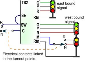
Contacts are shown in the "normal" position (N) with points set for the main track.
