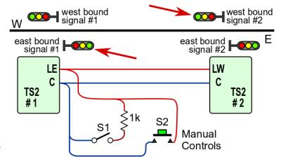
To manually clear an 'occupied' block, momentarily connect the 'Link' terminal (LE for the east side, or LW for the west
