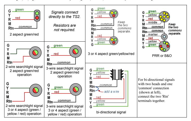
Note that **resistors** are **not** required because resistors are built in to the TS2 circuit board.
