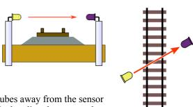
**Tip #1** - If mounting the sensors vertically as shown here, slide the plastic tubes away from the sensor then carefully bend the leads to a right angle. The leads are somewhat brittle, bending them more than two or three times may cause a break.
