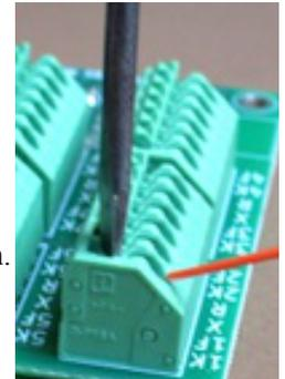
**Connect sensor pair 1:** Connect the orange (or red) wire from the IR LED to terminal 1K. Connect the green (or blue) wire from the IR photo receiver to terminal 1F. Now, how you connect the two white (or yellow) wires to the MRD6T will determine whether Detector 1 will operate in 'Across the Track' or 'Reflective' mode. See the diagrams below.
