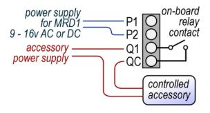
The MRD1's contact is rated for up to 3 amps and up to 28 volts. For higher power loads, use the MRD1 to control a power relay, such as the Azatrax MRAPR, then use the contacts of the power relay to switch the load.
