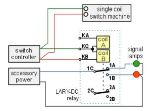
The DPDT contacts can be wired to a DC motor. This allows the motor direction to be controlled by two momentary push buttons.
